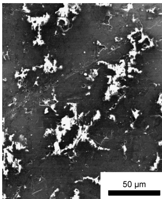
Fig. 6. SEM image of the test specimen after the continuous test under N_2 atmosphere.
